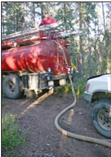
Hoselines were connected and run down to the pump. We used a length of 4" suction, 4 lengths of 4" supply line, the manifold, and 1 length of 2 1/2" to reach the tanker from the lake.
